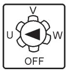
Figure 19. AC Ammeter Change-Over Switch
